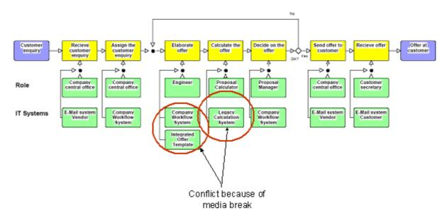
The process indicates also the relevant roles in the enterprises that are involved into the process execution. Information breaks can also be analysed in detail by showing the properties of the currently not interoperable systems.
